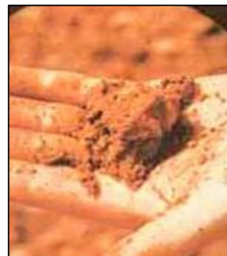
Close to optimum and ready for compaction
